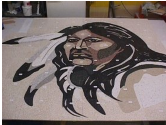
School logo completely fabricated using KMT Waterjet to meet the Oak Grove High School Administrators' requirements for lobby floor "school logo" decoration.
